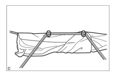
(3) Position the front seat airbag assembly inside the tire with the airbag deployment side facing inward.
