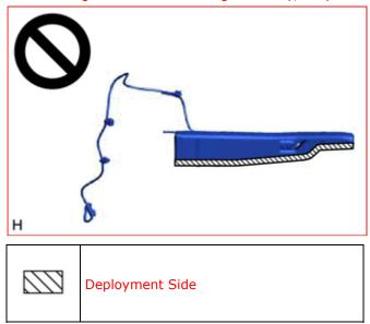
(c) Using braided wire, tie down the front seat airbag assembly to an unneeded tire.
