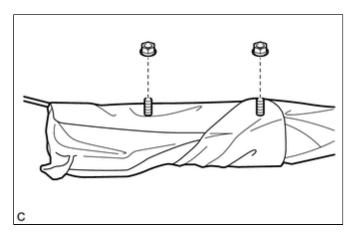
(2) Wind 2 or more wires around the stud bolts of the front seat airbag assembly as shown in the illustration.
