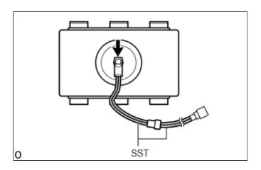
(d) Using braided wire, tie down the instrument panel passenger airbag assembly to an unneeded tire.
