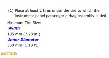
Do not place the SST connector under the tire because it could be damaged.
