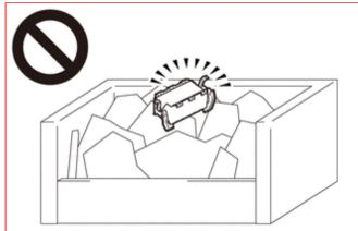
• The airbag produces an exploding sound when it is deployed, so perform the operation outdoors where it will not disturb nearby residents.
