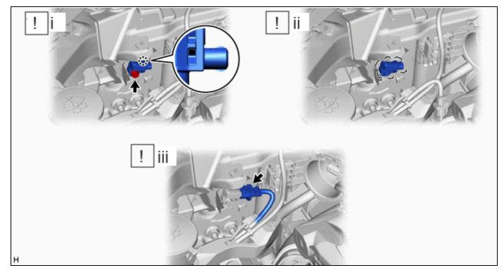
(1) Engage the claw and install the front airbag sensor with the bolt.
