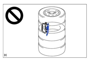
(1) Place at least 2 tires under the tire to which the curtain shield airbag assembly is tied.
