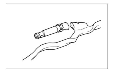
(d) Using braided wire, tie down the curtain shield airbag assembly to an unneeded tire.
