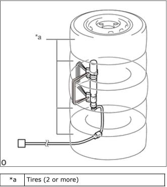
(2) Place at least 2 tires onto the tire to which the curtain shield airbag assembly is tied. The top tire should have a wheel installed.
