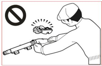
• Do not apply water, etc. to a curtain shield airbag assembly with a deployed airbag.
