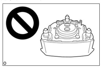
(b) When storing the airbag, do not place anything on top of the airbag or pile up airbags.
