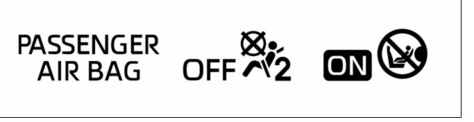
(3) Approximately 6 seconds after the ignition switch is turned to ON, the passenger airbag ON/OFF indicator will indicate ON/OFF depending on the following conditions.
