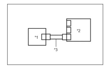
(a) Connect the airbag ECU assembly connector.
