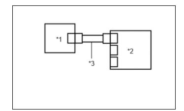
(a) Connect the airbag ECU assembly connector.
