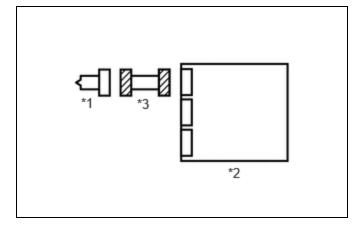
(a) Disconnect the airbag ECU assembly connector.
