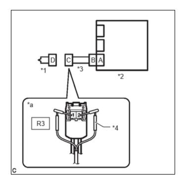
(a) Connect the airbag ECU assembly connector.
