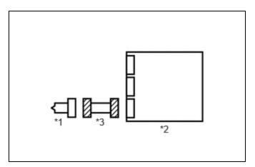
(a) Disconnect the airbag ECU assembly connector.
