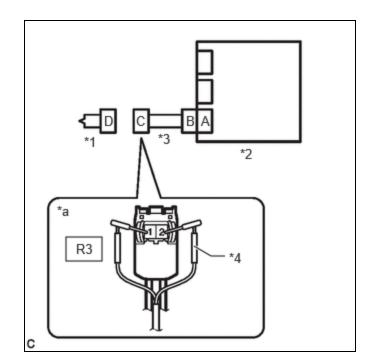
(a) Connect the airbag ECU assembly connector.
