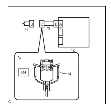
(a) Connect the airbag ECU assembly connector.
