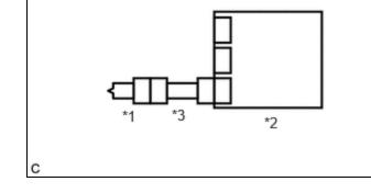
(a) Connect the airbag ECU assembly connector.
