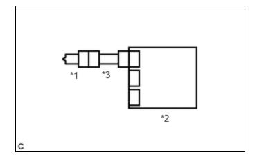
(a) Connect the airbag ECU assembly connector.
