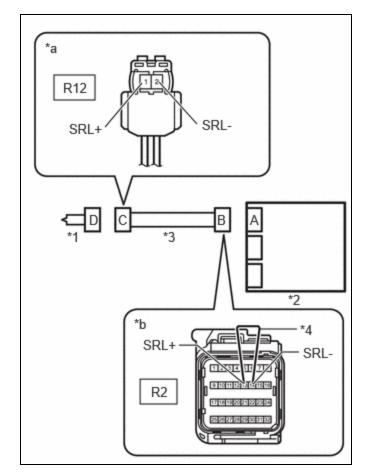
(a) Disconnect the airbag ECU assembly connector.
