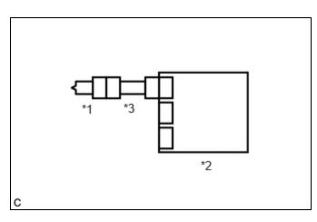
(a) Connect the airbag ECU assembly connector.
