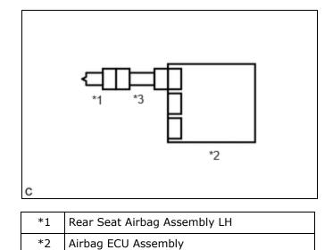
(a) Connect the airbag ECU assembly connector.
