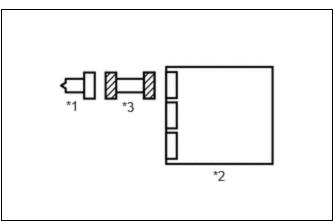
(a) Disconnect the airbag ECU assembly connector.
