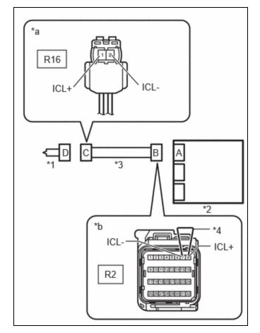
(a) Disconnect the airbag ECU assembly connector.
