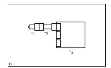
(a) Connect the airbag ECU assembly connector.
