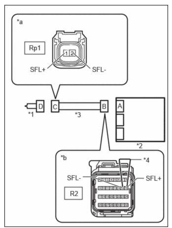
(a) Disconnect the airbag ECU assembly connector.
