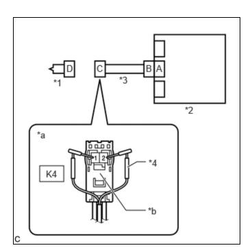
(a) Connect the airbag ECU assembly connector.
