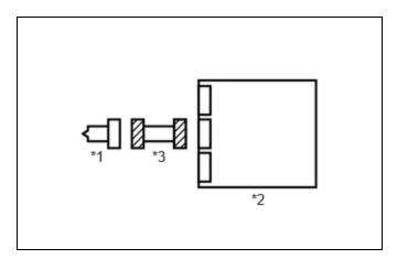
(a) Disconnect the airbag ECU assembly connector.
