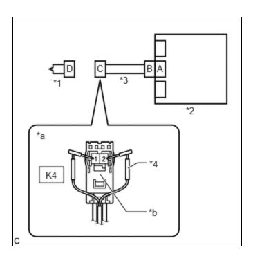
(a) Connect the airbag ECU assembly connector.
