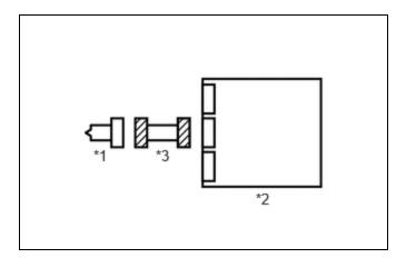
(a) Disconnect the airbag ECU assembly connector.
