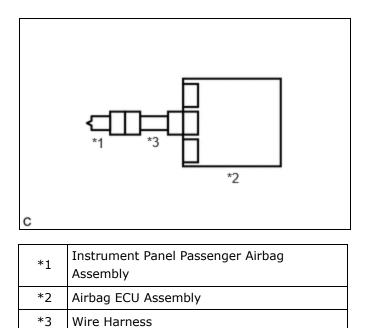
(a) Connect the airbag ECU assembly connector.
