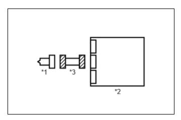
(a) Disconnect the airbag ECU assembly connector.
