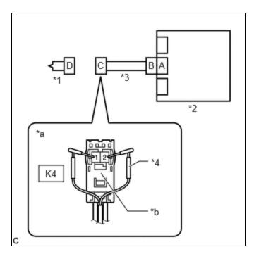
(a) Connect the airbag ECU assembly connector.
