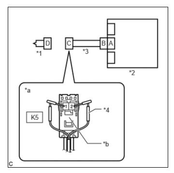
(a) Connect the airbag ECU assembly connector.
