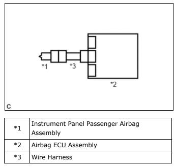
(b) Connect the instrument panel passenger airbag assembly connector.
