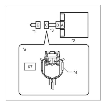
(a) Connect the airbag ECU assembly connector.
