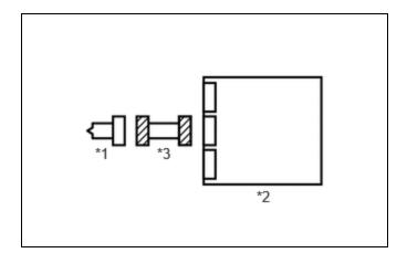
(a) Disconnect the airbag ECU assembly connector.
