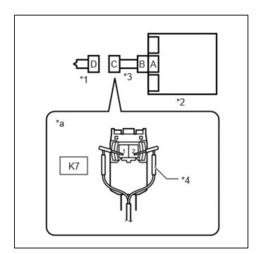
(a) Connect the airbag ECU assembly connector.
