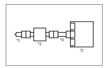
(a) Connect the airbag ECU assembly connector.
