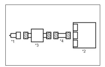
(a) Disconnect the airbag ECU assembly connector.
