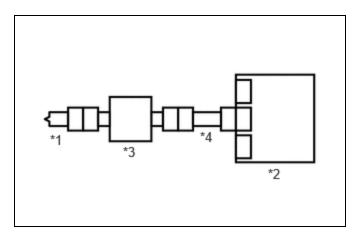
(a) Connect the airbag ECU assembly connector.
