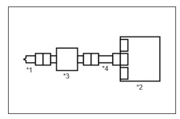
(a) Connect the airbag ECU assembly connector.
