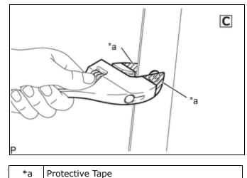
(c) When the adjustment screw of the adjustable wrench can no longer be turned by hand, tighten
