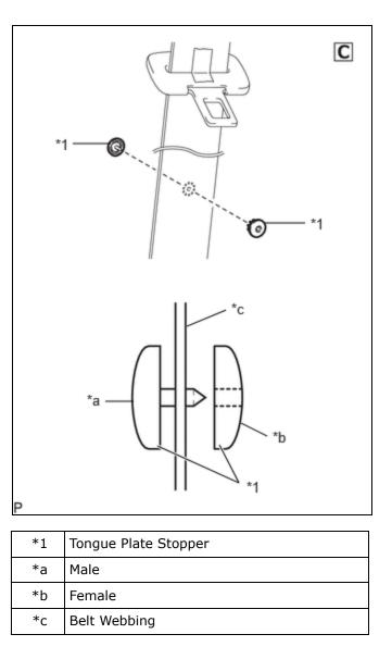
(b) Hold the tongue plate stopper in the hole of the belt webbing using an adjustable wrench, and turn the adjustment screw of the adjustable wrench by hand to compress the tongue plate stopper.
