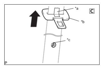
(a) Slide the tongue plate above the installation position of the tongue plate stopper, and temporarily hold it with adhesive tape.
