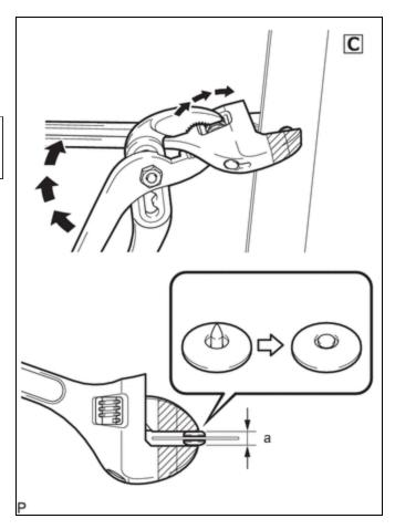
(d) Make sure that the pin of male side of the tongue plate stopper has expanded evenly in the hole of the female part and is firmly held to the belt webbing. (Refer to the illustrations.)
