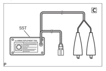
When deploying a seat belt pretensioner, always use the specified SST.
