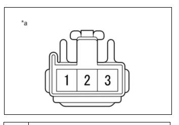
\*a Component without harness connected (Front Seatback Heater Assembly LH)
