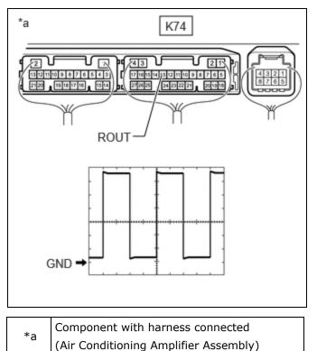
(a) Connect the K74 air conditioning amplifier assembly connector.
