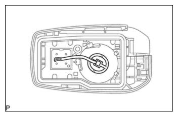
(3) Check the transmitter battery voltage.
