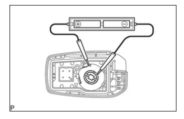
(3) From outside the vehicle, approximately 1 m (3.28 ft.) away from the driver door outside door handle, test the electrical key transmitter sub-assembly by pointing its key plate at the vehicle and pressing an electrical key transmitter sub-assembly switch.
