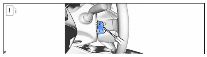
(1) Using a screwdriver with its tip wrapped with protective tape, disengage the 2 claws and 2 guides to remove the No. 3 steering wheel lower cover as shown in the illustration.
