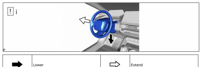
(1) Release the tilt and telescopic lever and fully extend and lower the steering column sub-assembly.
