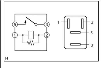
If the result is not as specified, replace the windshield wiper relay.
