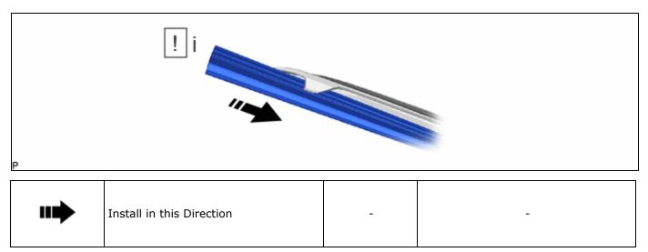
(1) Install the wiper rubber with the front wiper rubber backing plates to the front wiper blade as shown in the illustration.
