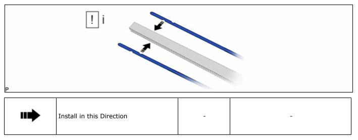
(1) Install the 2 front wiper rubber backing plates to the wiper rubber as shown in the illustration.
