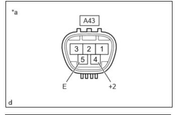
\*a Component without harness connected (Windshield Wiper Motor Assembly)
