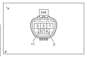
\*a Component without harness connected (Windshield Wiper Motor Assembly)
