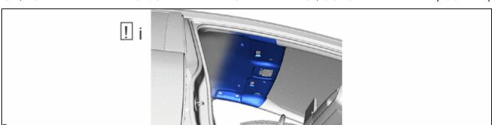
(1) Return the front section of the roof headlining assembly to its original position.
