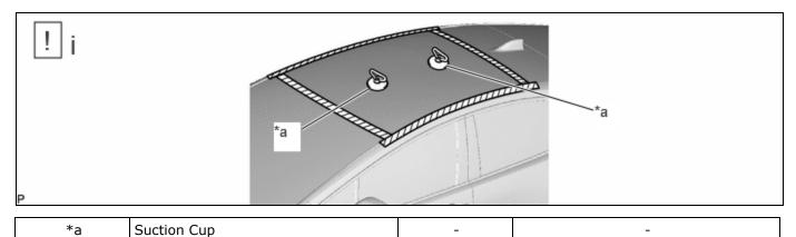
(1) Install the 2 suction cups to the No. 1 roof window glass sub-assembly.
