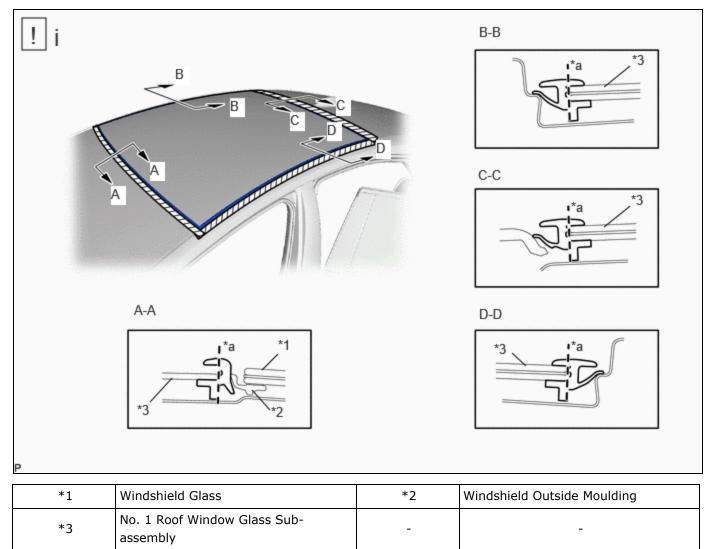
(1) Using a knife, cut off the roof window upper moulding as shown in the illustration.
