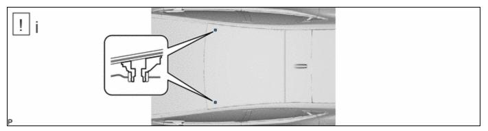
(1) Using 2 suction cups, remove the No. 1 roof window glass sub-assembly.
