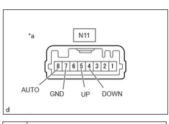
\*a Component without harness connected (Power Window Regulator Switch Assembly)
