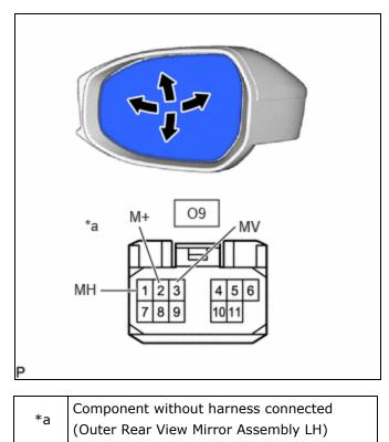
(1) Disconnect the outer rear view mirror assembly LH connector.
