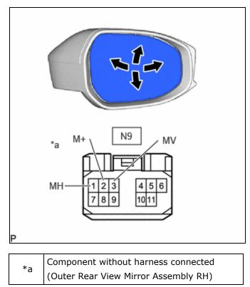
(1) Disconnect the outer rear view mirror assembly RH connector.
