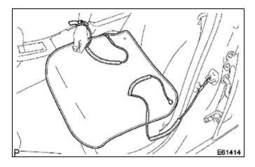
(d) Connect SST (No. 1 grounding wire), SST (wristband) and SST (anti-static mat).
