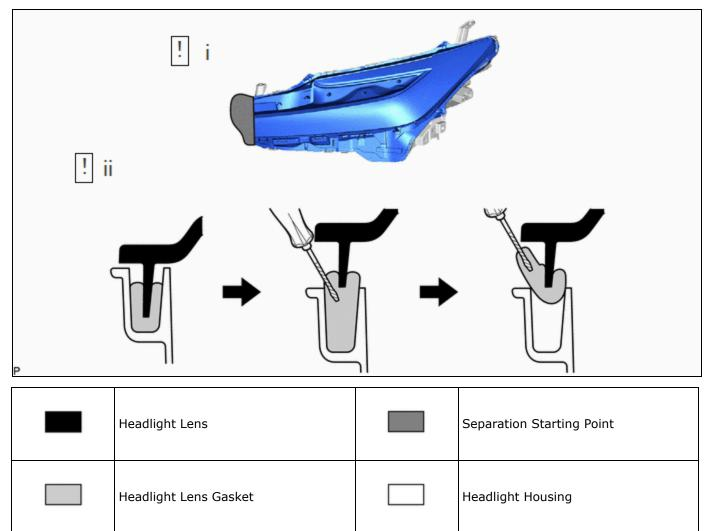
(1) Insert a finger between the headlight lens and headlight housing and lift up the headlight lens.
