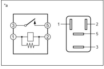
\*a Component without harness connected (HORN Relay)
