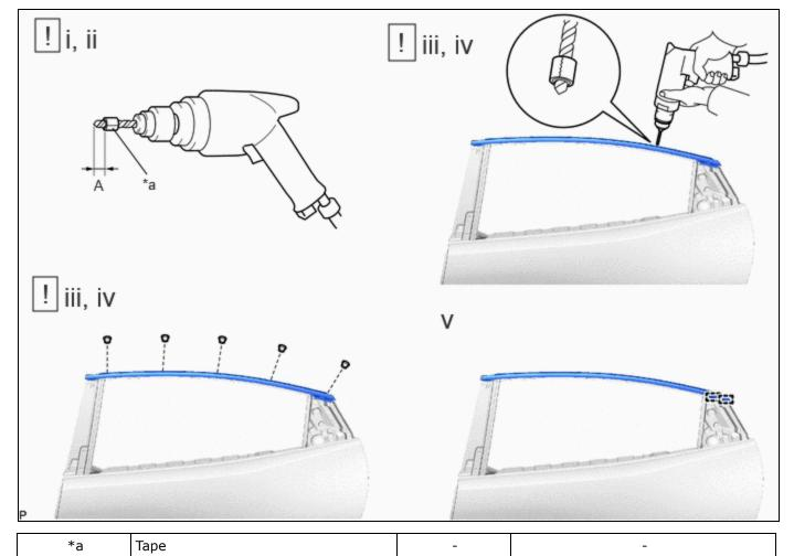
(1) Insert a 4.0 mm (0.157 in.) drill bit into a drill.
