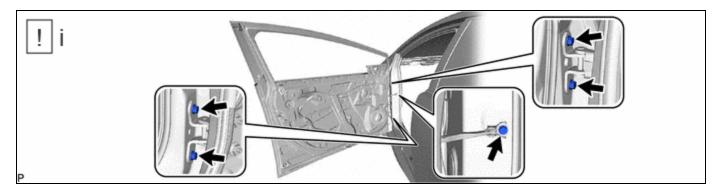
(1) Remove the 5 bolts and front door panel sub-assembly.
