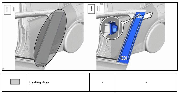
(1) Using a heat light, heat the vehicle body and front door window frame rear moulding surface.
