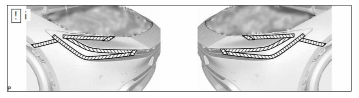
(1) Apply protective tape around the front bumper assembly as shown in the illustration.
