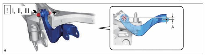
(1) Temporarily install the rear upper control arm assembly LH to the rear suspension member sub-assembly with the bolt and nut.
