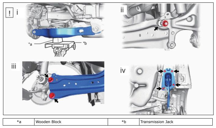
(1) Using a transmission jack and a wooden block, support the rear No. 2 suspension arm assembly.
