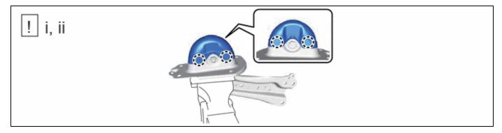
(1) Secure the rear trailing arm assembly in a vise using aluminum plates.
