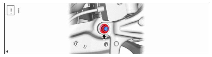
(1) Remove the nut and rear stabilizer link assembly LH from the rear trailing arm assembly.
